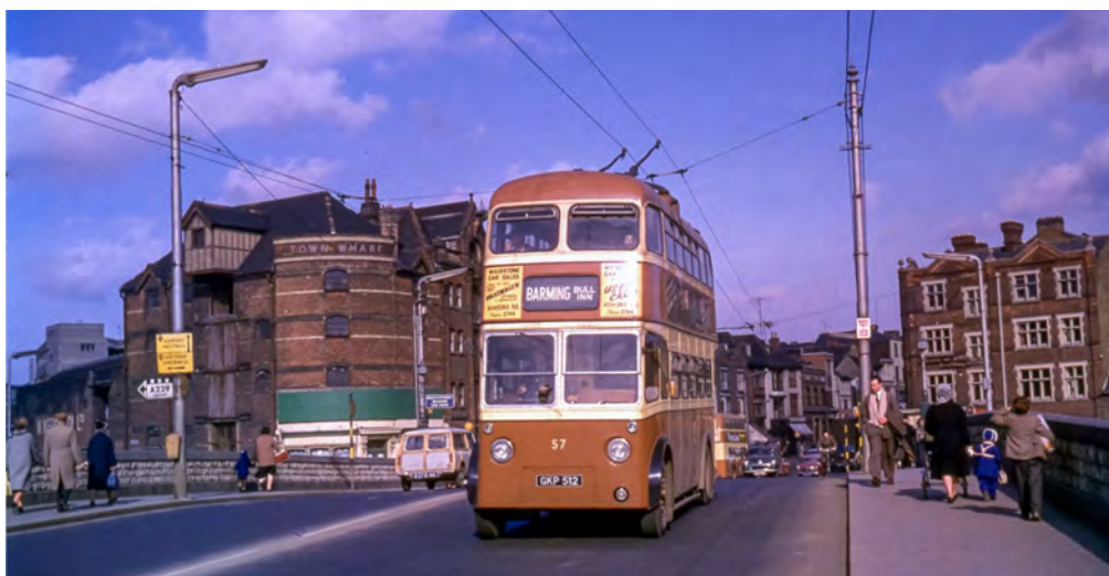
Above: Huddersfield: Roe re-bodied Karrier trolleybuses meet at the Slaithwaite 'Birks Well' short working turning circle (service 41). On the left, Roe re-bodied pre-war Karrier E6 number 492 is proceeding to the terminus of the route at Marsden (service 40). On the turning circle is 568, a post-war Karrier-badged Sunbeam MS2 which was given a new body by Roe in 1958. Almost all of the Marsden route was along the A62 trunk road between Yorkshire and Lancashire, and the relatively wide road has allowed the baby Austin car to overtake. 7 September 1962
