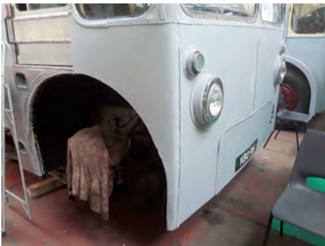
Cardiff 243 offside panel renewed, then given a coat of grey etched primer. [Keith Walker]
