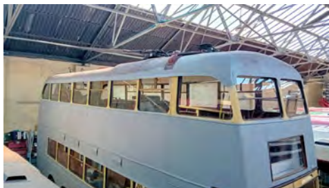
All the horizontal half-round beading now fitted to the offside of Cardiff 262. [Keith Walker]
