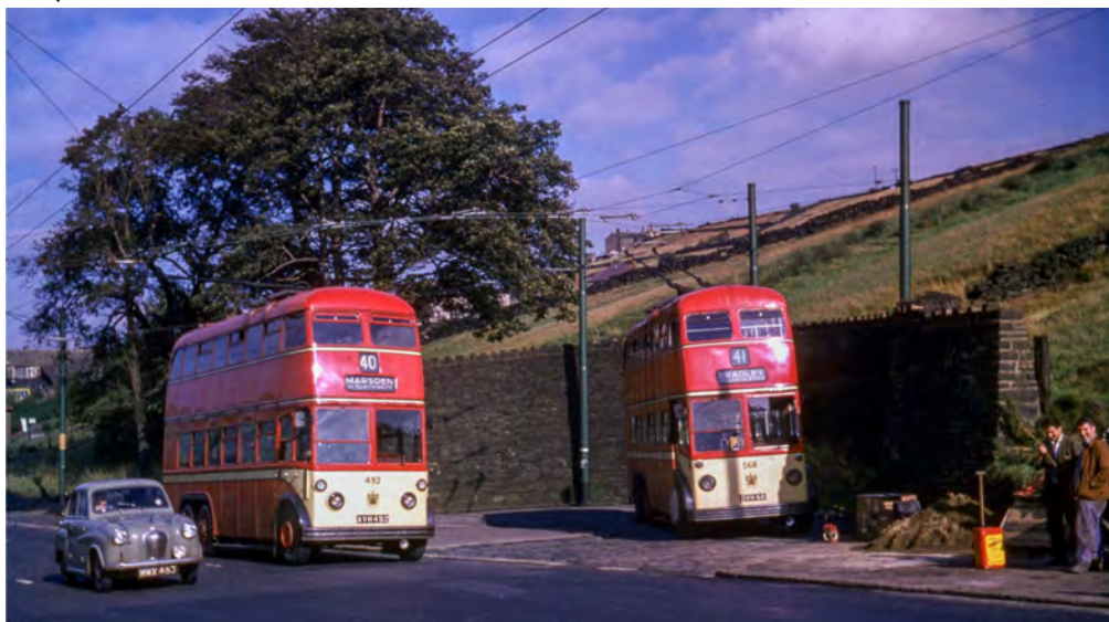
Above: Huddersfield: Roe re-bodied Karrier trolleybuses meet at the Slaithwaite 'Birks Well' short working turning circle (service 41). On the left, Roe re-bodied pre-war Karrier E6 number 492 is proceeding to the terminus of the route at Marsden (service 40). On the turning circle is 568, a post-war Karrier-badged Sunbeam MS2 which was given a new body by Roe in 1958. Almost all of the Marsden route was along the A62 trunk road between Yorkshire and Lancashire, and the relatively wide road has allowed the baby Austin car to overtake. 7 September 1962
